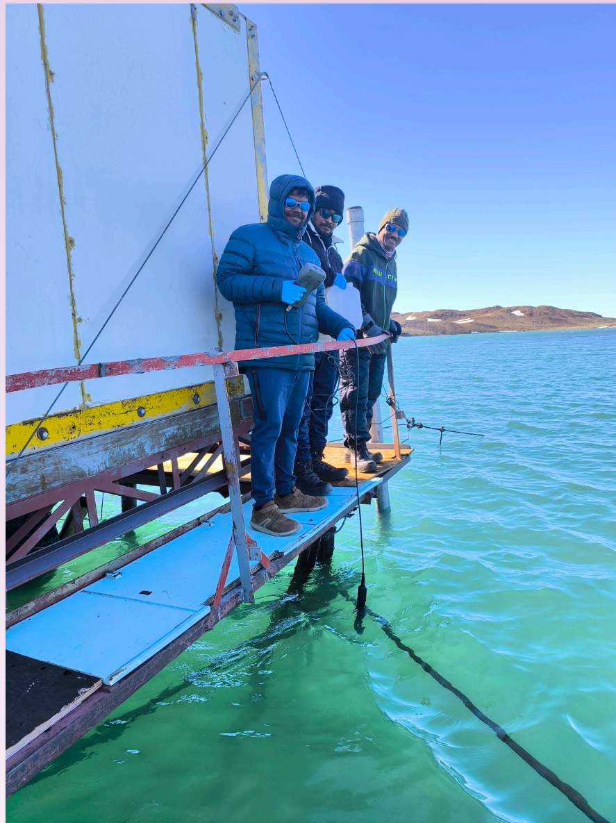
Fig. 7. Measurement of water column parameters in the Priyadarshini Lake from a platform near the Maitri research station using a water-quality probe.
