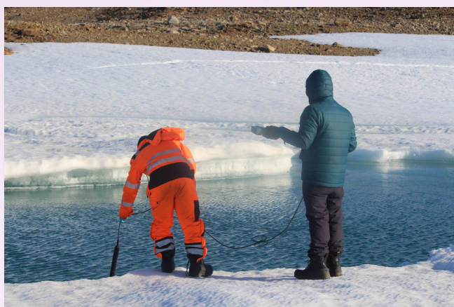
Fig. 1. Field team (Dr. Srinivas Bikkina & Dr. Manoj MC) measuring lake water parameters using a multiparameter probe in a partially frozen Antarctic Lake during sampling operations.
